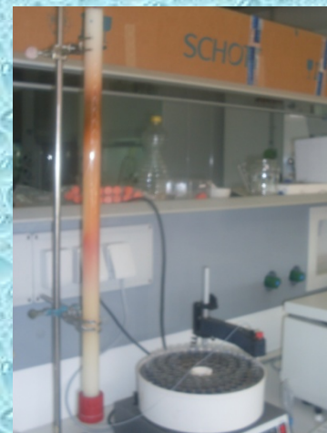
Isolation of crude methanolic extract of NG Propolis using sephadex LH-20 on column
